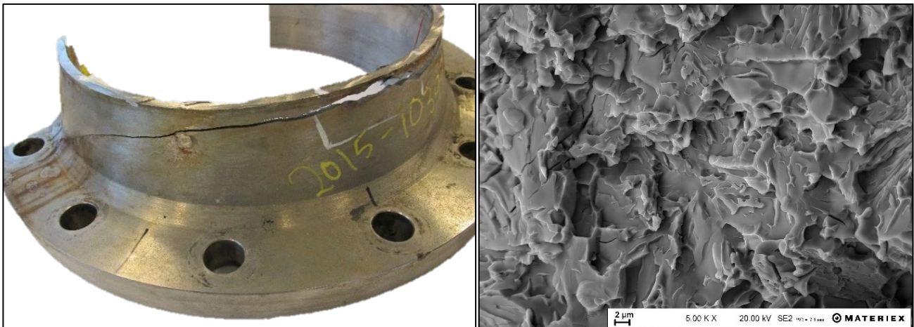
Figure 2. Left: cracked flange. Right: SEM-image of fracture surface showing a brittle cleavage mode of fracture.
